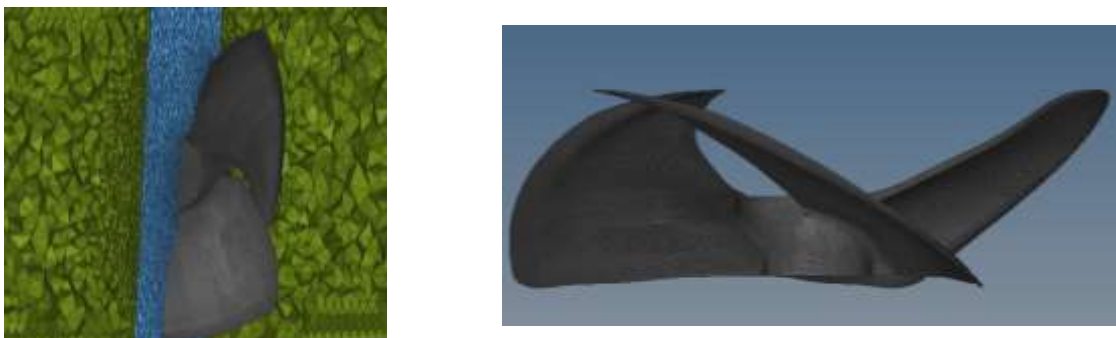
Fig4: Computational mesh on the fan blade and fluid domain
